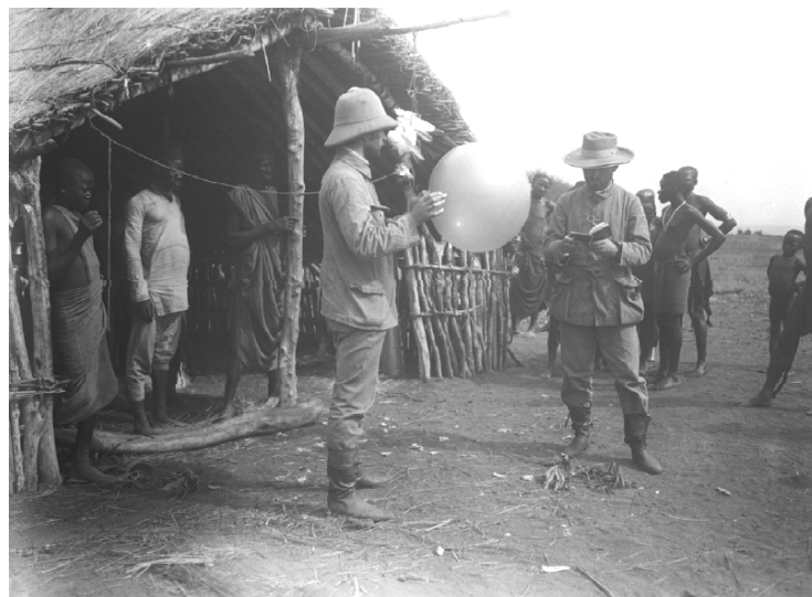
FIGURE 2 Colonial data form part of current products on which decisions are based. German aerologists in the East African colonies in 1908, measuring vertical wind profiles using balloons (Brönnimann and Stickler, 2013, photo provided by Hans Steinhagen, Lindenberg)
