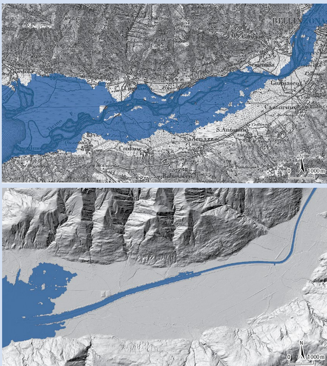
Fig. 52: Comparison of the floodplains from the reconstructed flood event of 1868 (top) and the simulated effects of the same event under today's conditions (bottom).
